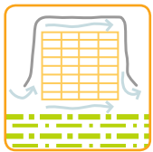
Ventilation under presenning
